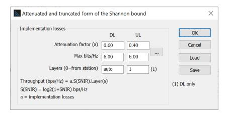
S(SNIR) = Shannon bound, which represents the maximum theoretical throughput that can be achieved over an AWGN (Additive White Gaussian Noise) channel with a given SNR. a = attenuation factor of the Shannon bound (implementation losses).
