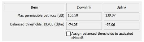
**Assign balanced thresholds to activated eNodeB:** If checked, this option will update the coverage and receiving thresholds parameters of the activated stations with the balanced values found.
