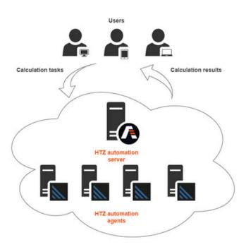
HTZ Automation features a client-server architecture with requests managed through HTTP or other secure modes. Other architectures like Web Socket can also be accommodated. All options offer a high-level of interoperability and functions can be plugged-in to meet end user requirements.
